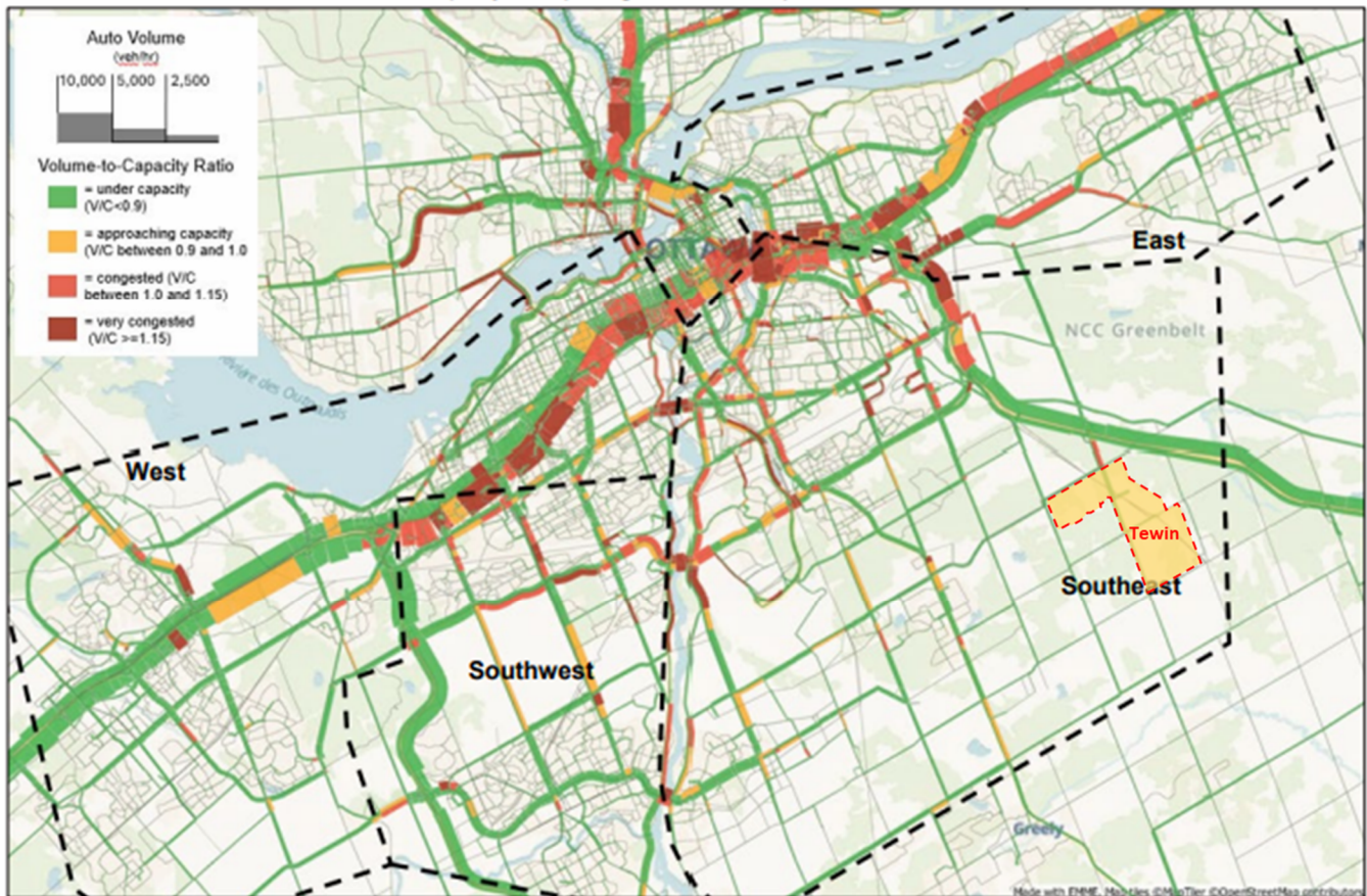
Figure 28: TMP EMME 2046 Auto Volume-to-Capacity Ratios (AM Peak Hour, 16,000 Official Plan Base Case Scenario)
